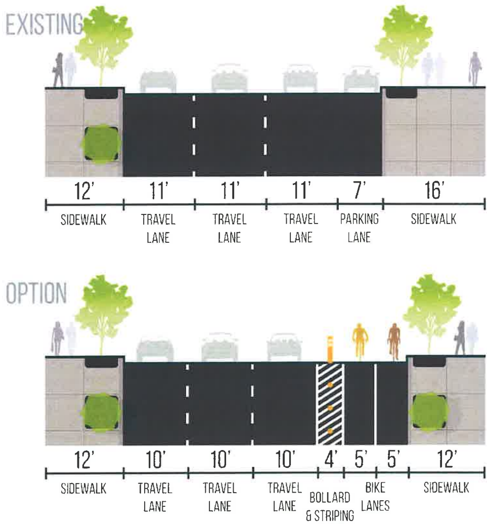
Figure 60 Conceptual cross section for Walnut Street at 10th Street Source: Sam Schwartz / Interface Studio
