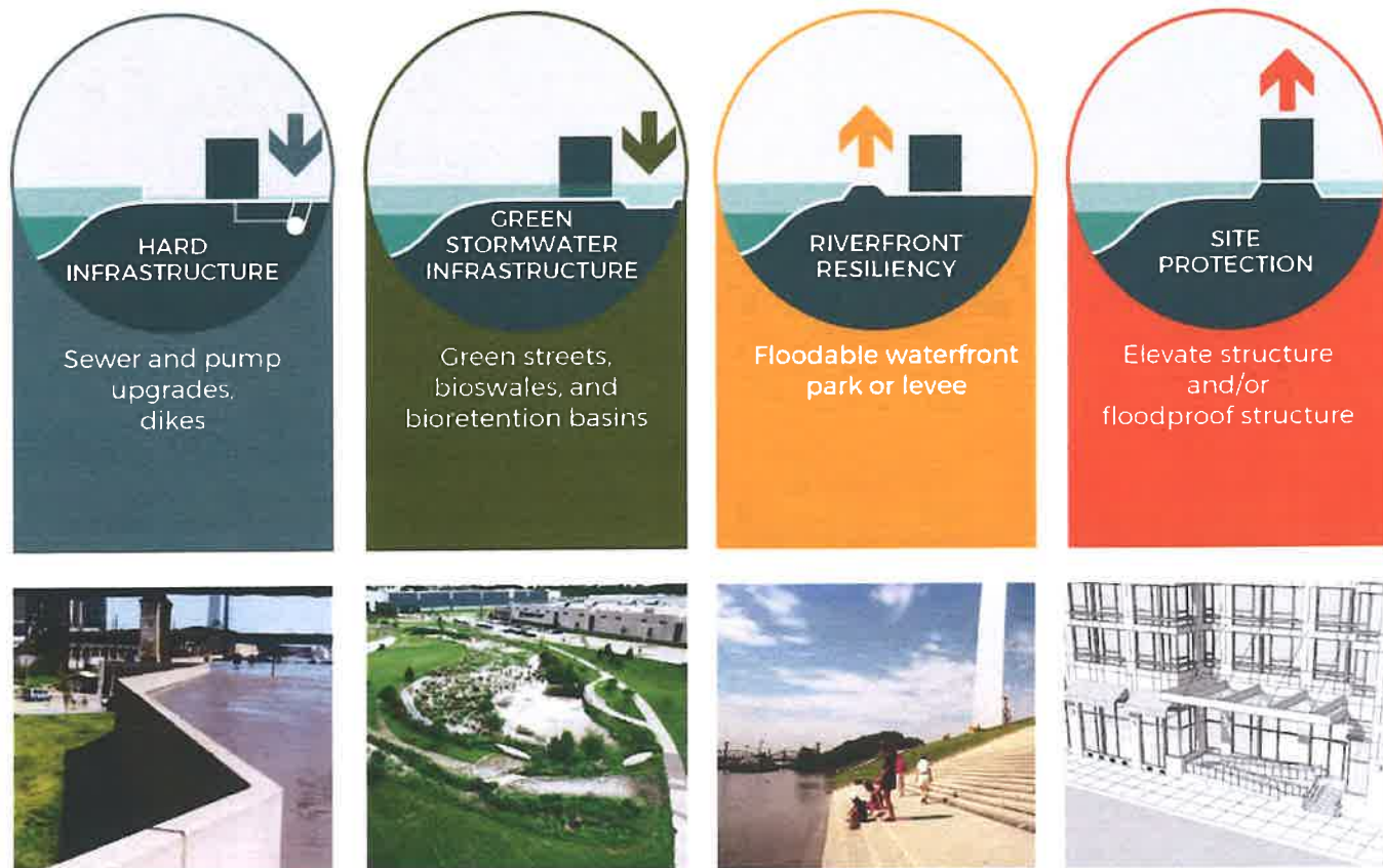
Figure 71 Flood and sea level rise resilience measures
